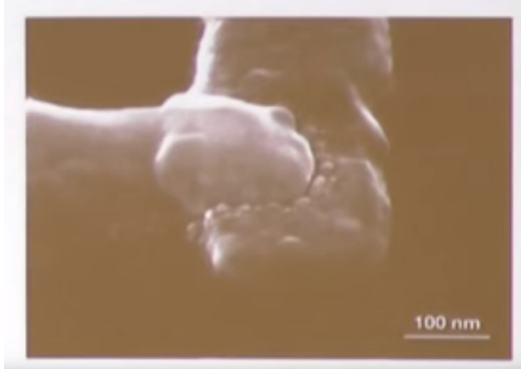
Figure 4a: A real Josephson Junction. These are fabricated by oxidising an Aluminium wire and then laying another Aluminium wire above. Fortunately the oxidation of Aluminium is a self-terminating process, and the height at which the process stops is appropriate for the fabrication of Josephson Junctions. Source: Alexandre Blais.
